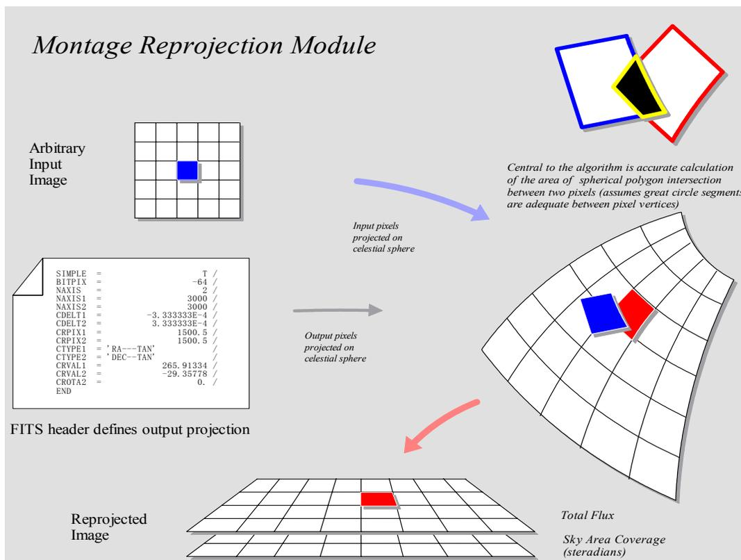
**Figure 4:** The Montage reprojection algorithm. This algorithm preserves the scientific fidelity and astrometric accuracy of the input images by employing spherical trigonometry to calculate the area of overlap between input and output pixels, and weighting the distribution of flux between input and output image by the areas of overlap.
