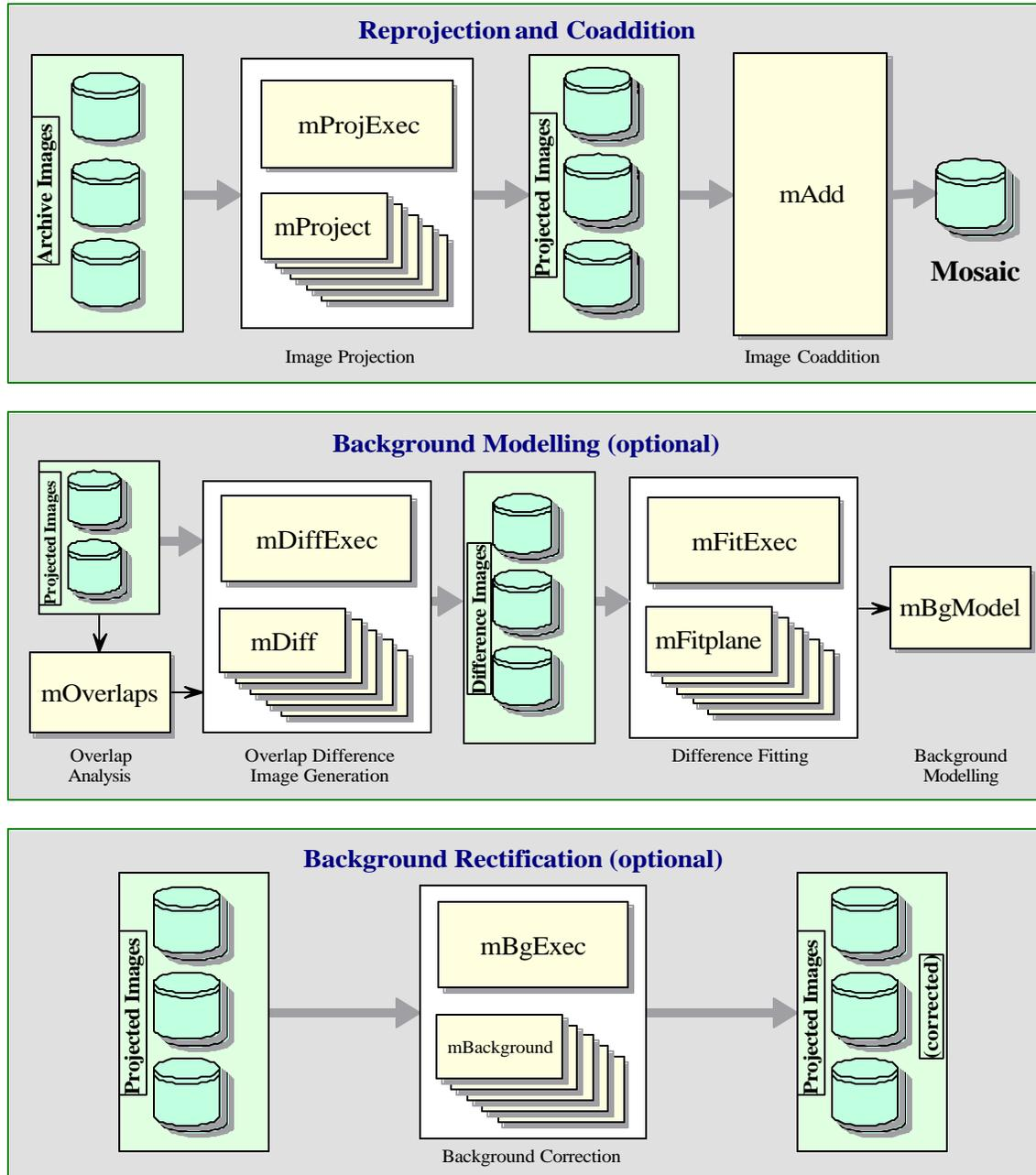
Figure 2: Design Components of Montage - Process Flow Overview.
